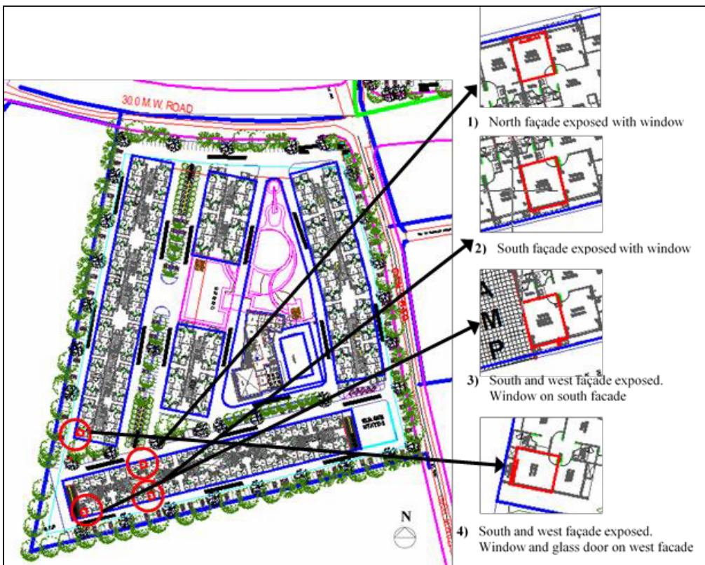
Figure 2: Site plan of Project 1, Indore. The 4 bedrooms selected for simulation are marked
