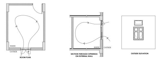
Addition of ventilator at an upper level increases the rate of convective heat exchange with the outside air.
