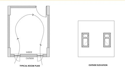
Figure 12 Two windows on single external wall (Guideline)
