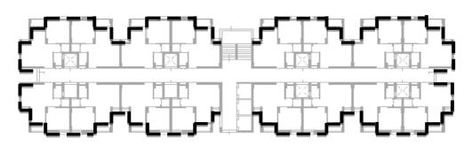
FIGURE 1 Walls included in the definition of building envelope
