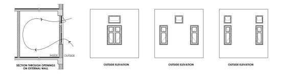
Figure 13 Adding ventilators above windows improves ventilation especially when only single external wall is available for openings (Guideline)
