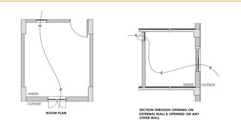
Figure 11 Openings on external wall and internal wall for cross ventilation (Guideline)
