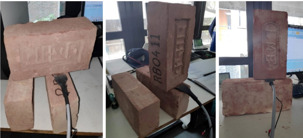
Figure-A2.5: Photographs demonstrating different combinations of brick specimens placed for measurement and hot disk probe sandwiched between two samples of firedclay brick.
