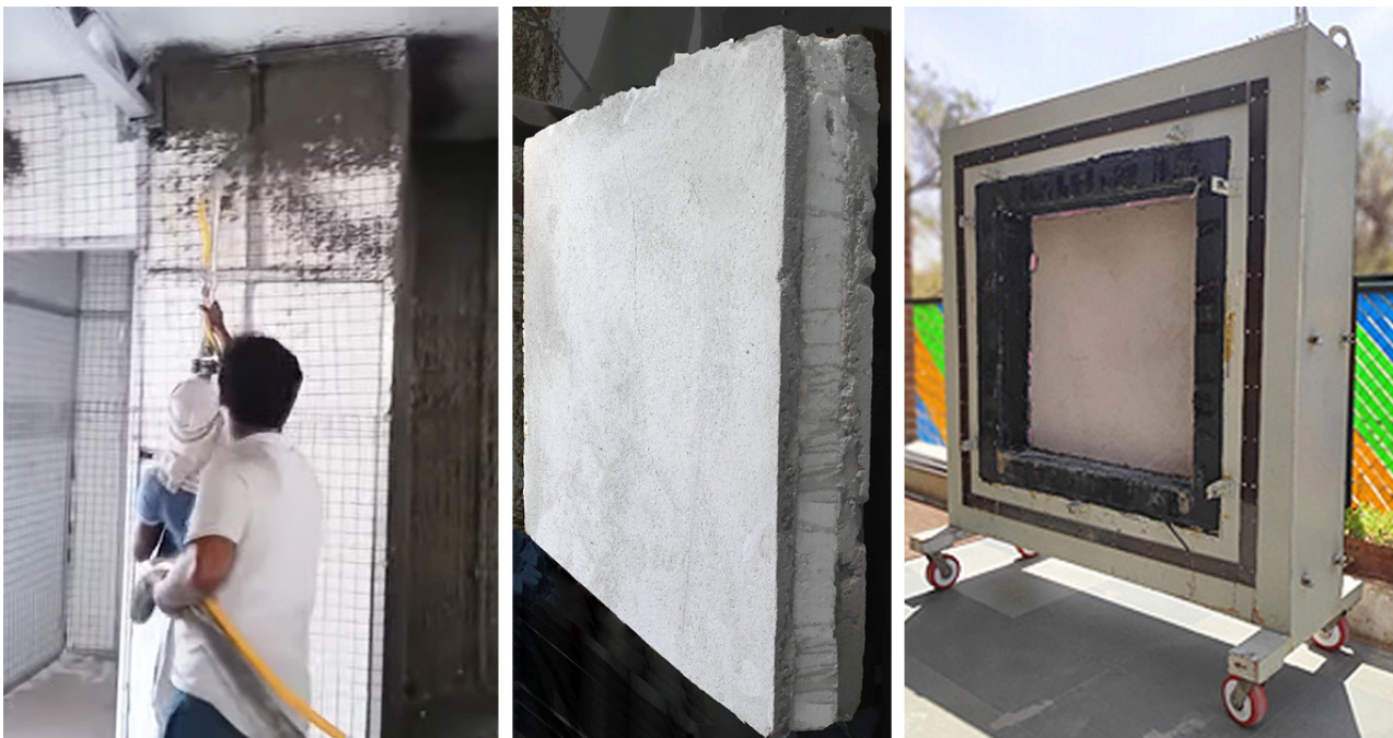
Figure 20: Example of on-site shotcreting (left), Sample of EPS core panel received from the manufacturer (middle) and EPS core panel fixed into the specimen frame of GHB(right)
