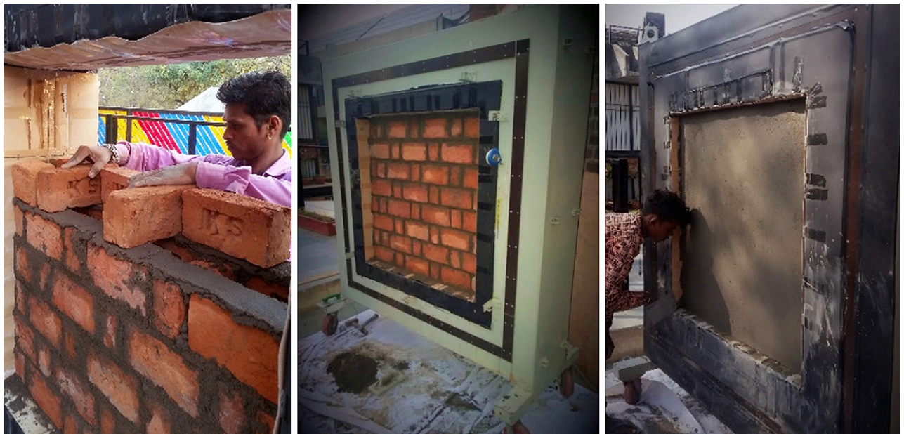
Figure 12: Photograph showing the construction of Rat-trap bond wall within the specimen frame of GHB.
