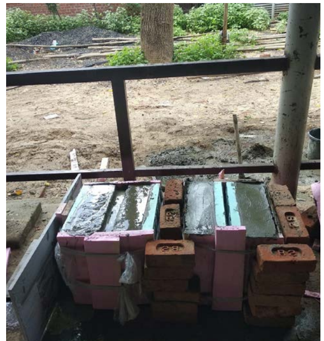
Figure 28: Photograph of an insulated coffer panel sample without concreting (left), Photograph of concrete poured in-situ in the insulated coffer panel sample (right). Source: (left) (BMTPC, 2018c)
