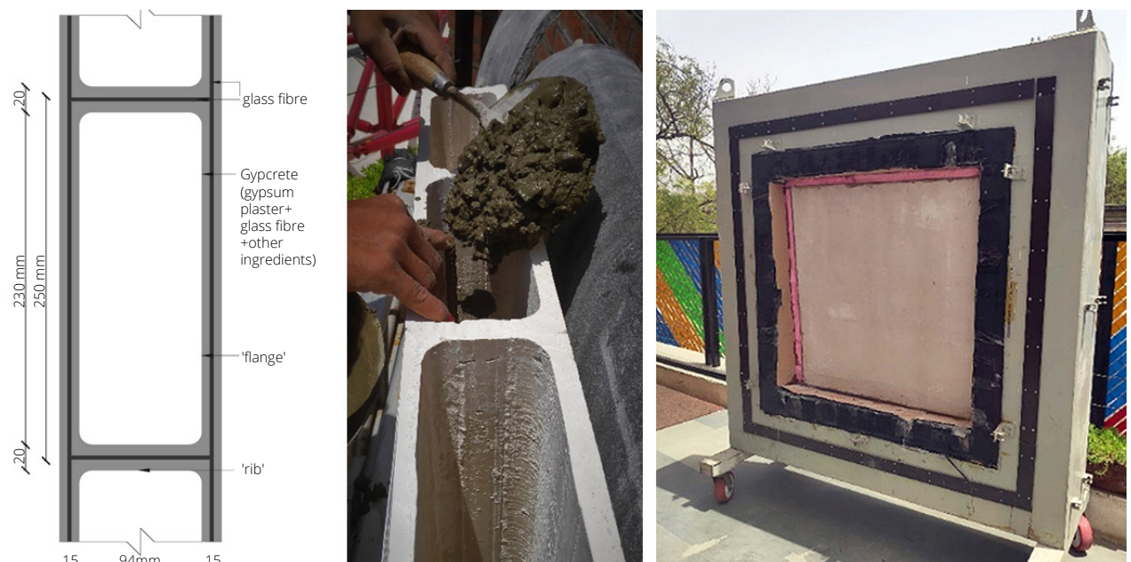
Figure 22: Components of a typical GFRG panel (left) (BMTPC, 2011), on-site preparation of GFRG partly filled panel (middle) and GFRG fully filled panel fixed into the GHB specimen frame (right)
