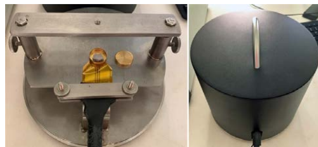
Figure-A2.10: Specific heat capacity measurement
