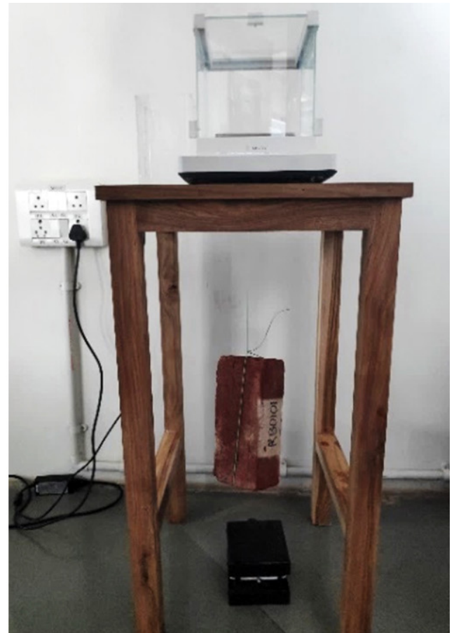
Figure-A2.14: Photograph showing measurement of suspended weight (S)(left) and saturated weight (W)(right) as per the procedure.
