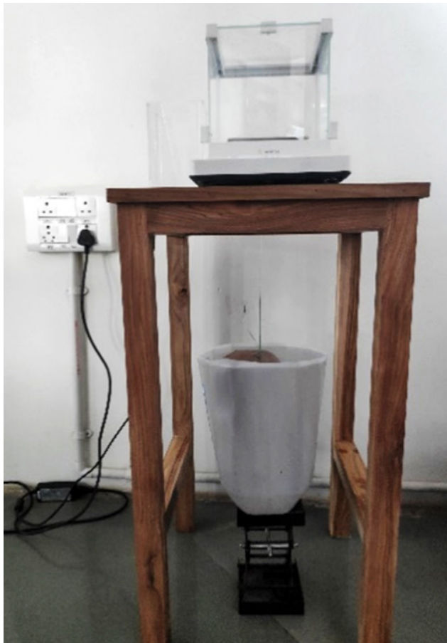
Figure-A2.14: Photograph showing measurement of suspended weight (S)(left) and saturated weight (W)(right) as per the procedure.
