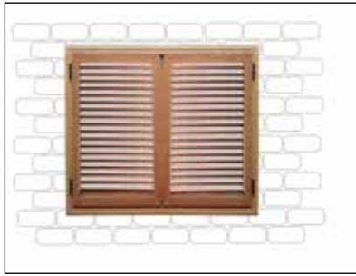
Fig. A: Shutter - Louvers at 0°
