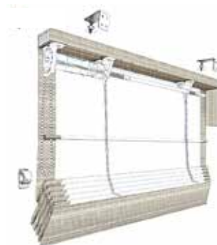
Fig. 2.4a: Components of Roman Fold Blind
