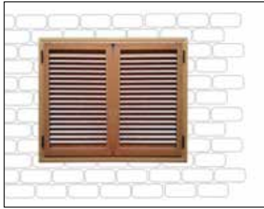
Fig. B: Shutter - Louvers at 45°
