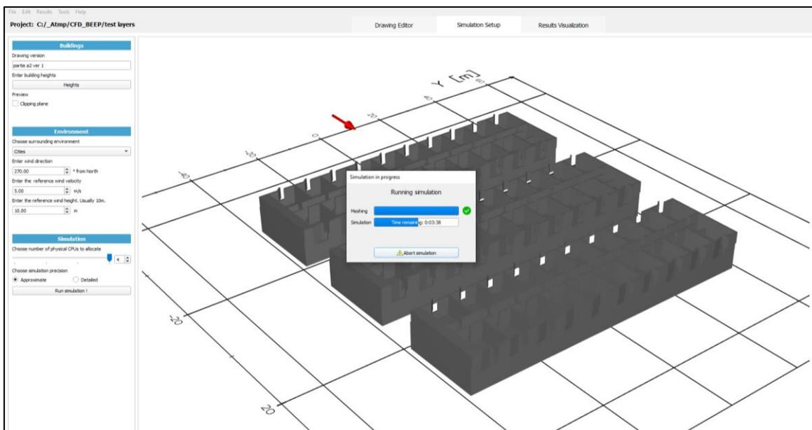
**Figure 3-29 Simulation running with estimation of remaining time (after meshing)**
