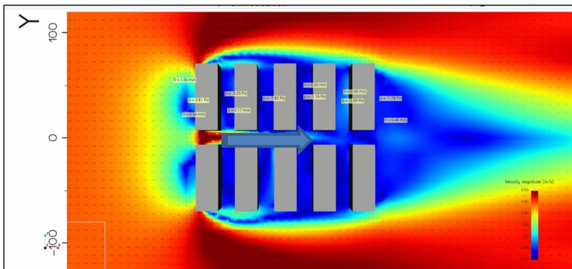
*Figure 5-1: buildings massing perpendicular to the wind direction*
