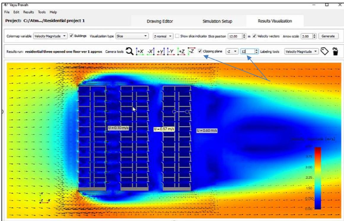
Figure 3-46 Without and with Clipped plane on Z axis
