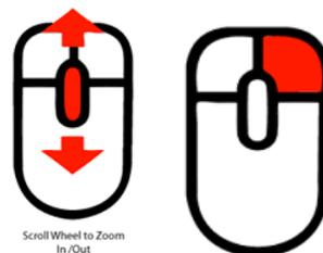
Zooming is obtained also by moving the mouse with the right button kept pushed (by sliding the mouse toward the screen)
