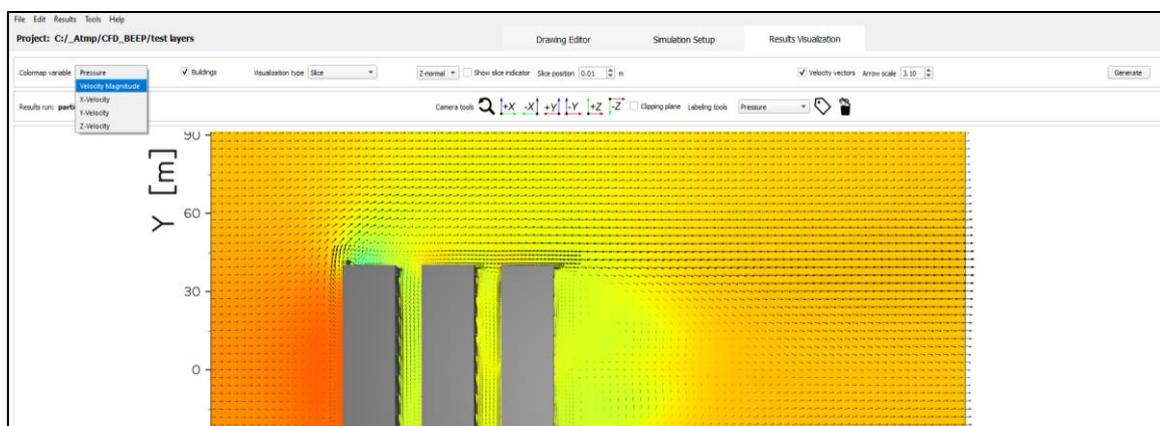
**Figure 3-33** Selecting the variable to analyze in simulation results
