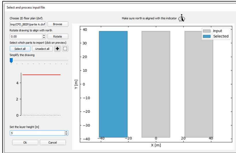
**Figure 3-8** The red line represents the height of the layer from the ground
