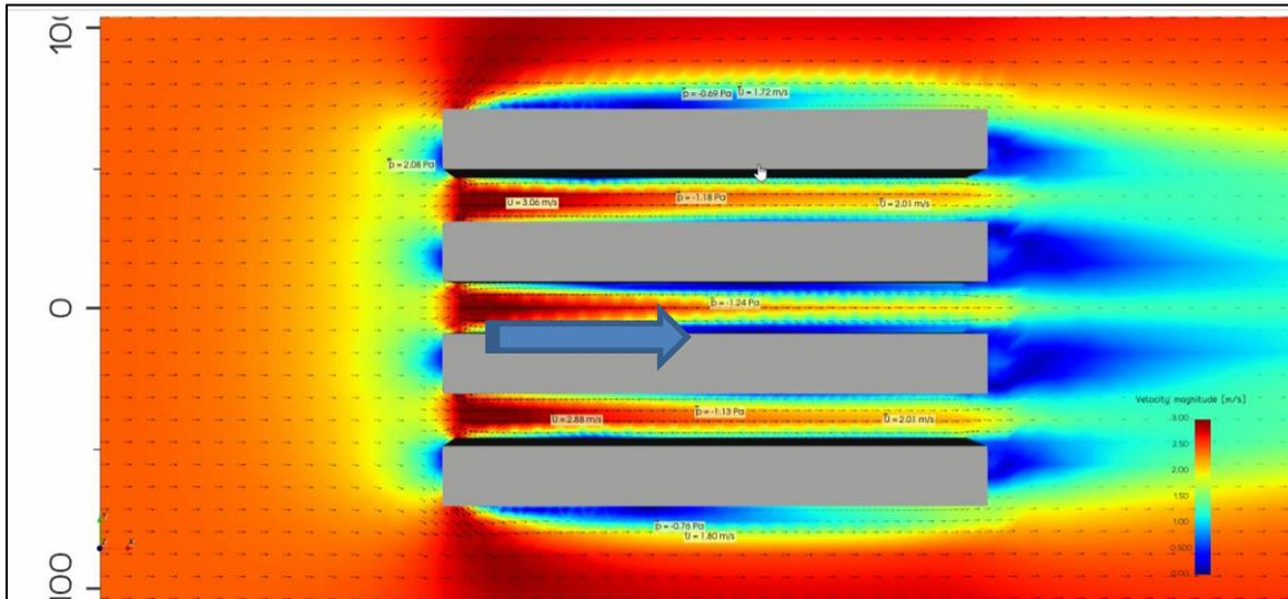
**Figure 5-2: long facades aligned with the wind direction**
