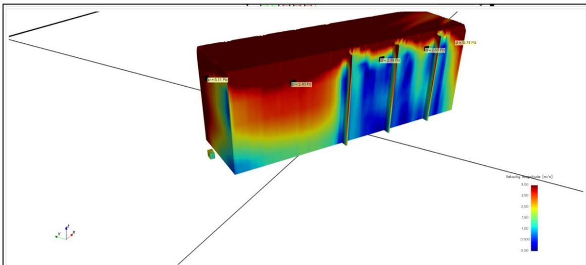
*Figure 4-2 Simulation results for building with closed flow*
