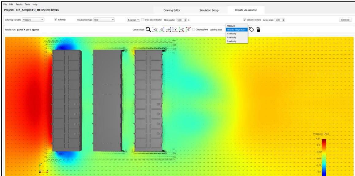
**Figure 3-41 Inserting quantitative labels in the simulation result**
