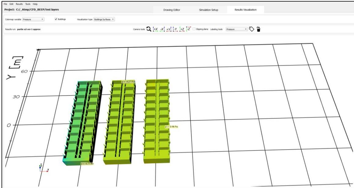
Figure 3-40 Building surface visualization, for viewing parameters at the building facade
