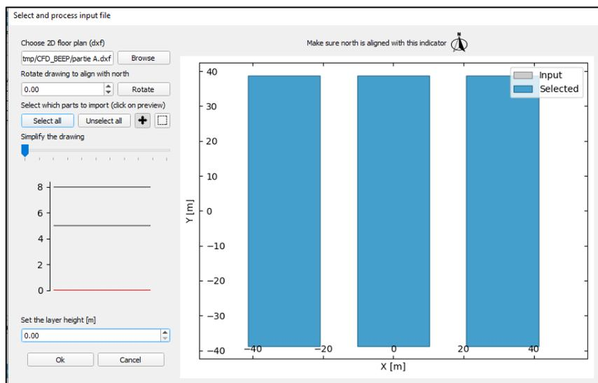
**Figure 3-9** Entering layer height (shown by the red line in the graph); all existing layers in the project are shown by black lines on the same graph
