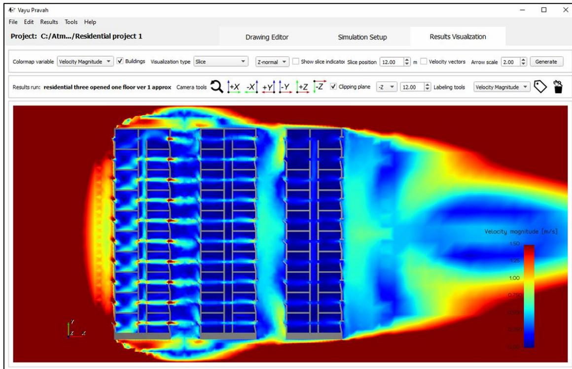
**Figure 5-3 Project with wind perpendicular to facade, simulation for wind velocity magnitude, slice at 12 m height**
