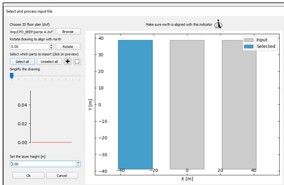
**Figure 3-7 Manually selecting part of the dxf to import in the plan**
