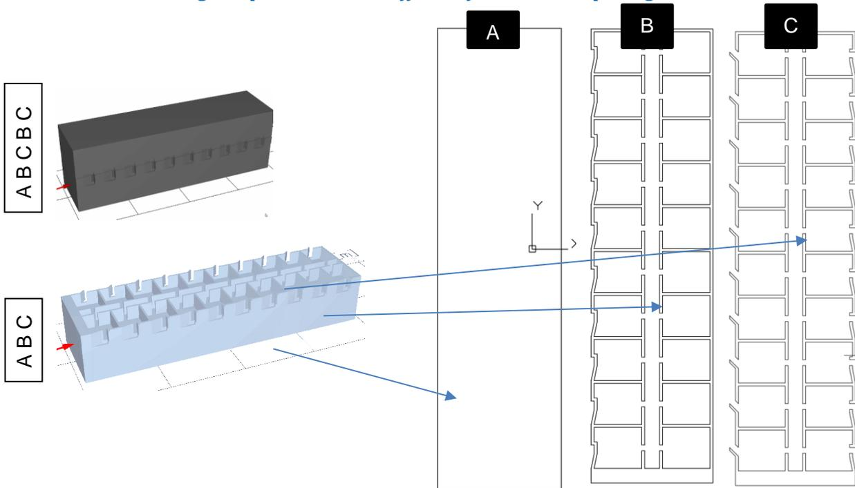
Figure 3-16 : façade profiles A) Bottom and top Rectangular closed façade profile B) closed façade with patterns C) open façade with aerodynamic elements
